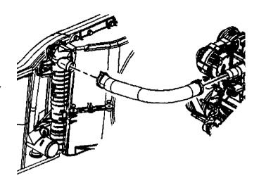
Remove air inlet and outlet hose, and battery junction box positive cable.
