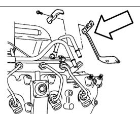
Remove the PCV hose and clamp from the driver and passenger side valve cover.
