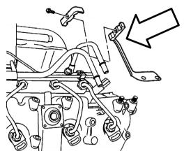
Reconnect the glow plug bracket, and connect the 24-pin and the 40-pin connectors.
