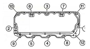
Clean lower valve rocker arm cover. Remove any sludge or other deposits. Clean lower valve rocker arm cover sealing surfaces. Inspect lower valve rocker arm cover for cracks or any damage. Inspect lower valve rocker arm cover sealing surfaces for damage. Replace lower valve rocker arm cover if any damage is found.
