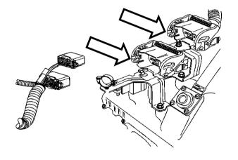
Reconnect the 3 glow plug relay on the driver side valve cover.
