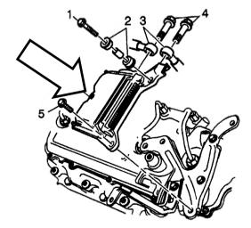
Disconnect and remove the fuel filter and housing.
