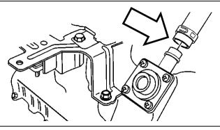
Reconnect fuel supply, return lines, and the L bracket. Tighten to 106 in. lbs. (12 N.m)
