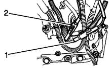
Connect the upper radiator hose, and fill coolant.
