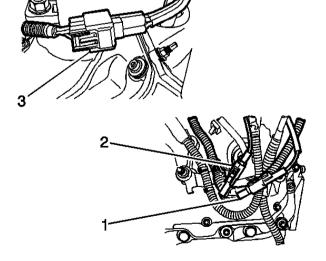
Remove the glow plug bracket, and disconnect both 40 and 24 pin engine connectors from the driver side valve cover.
