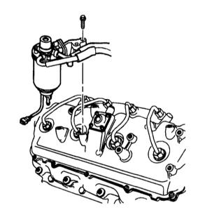
Install the FCIM to the passenger side cover with new seals. Tighten the bolts to:
