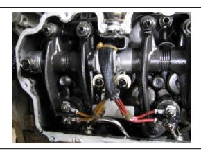
Remove 12 lower valve rocker arm cover bolts. Remove lower valve rocker arm cover. Remove gasket from lower valve rocker arm cover. Remove bolt grommets from lower valve rocker arm cover.
