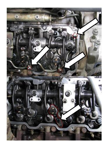
Remove the injector sleeves with GM Tool J-45910. If the injector sleeve was pulled from the cylinder head when removing the injectors.
