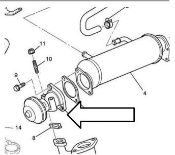
Remove water pipe outlet from the thermostat housing
