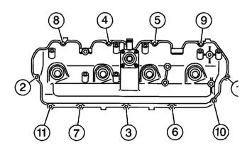
Clean upper valve rocker arm cover in suitable cleaning solvent. Inspect for cracking and other damage on upper valve rocker arm cover. Replace upper valve rocker arm cover if any damage.
