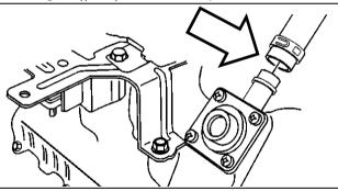
Remove the fuel injection control module (FCIM) from the passenger side valve cover.
